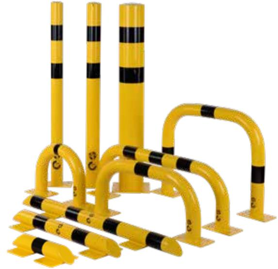
**Hoop protection guard, Ø 76 mm, galvanized and powder coated for outdoor use or powder coated for indoor use, yellow (like RAL 1023) with black warning stripes, material thickness 3,2 mm, base plate 120 x 195 mm, floor mounting via 8 drill holes Ø 12,5 mm, TÜV-certified (compliant with DGUV 108-007 / previously BGR 234).**
